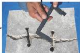
Our Staple System is made from 14 gauge steel, and because the staple is 90°, it gives extra strength so it will not bend out.
